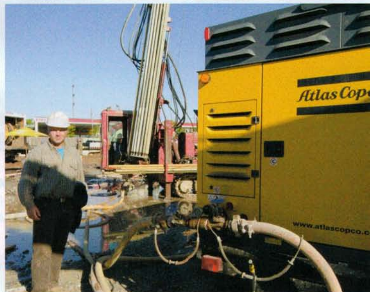
Stanley Reitsma stands next to the Atlas Copco XRVS 1000 CD6 compressor that is providing air to two drill rigs.
